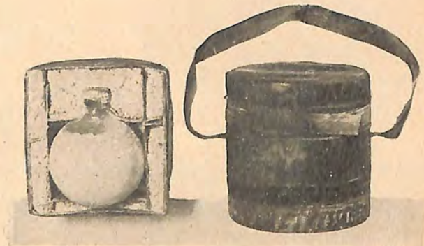
Figure 204. Frangible hydrocyanic acid grenade, arsenic trichloride stabilized type.
